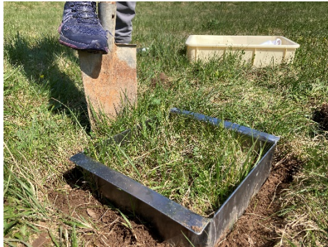
Fig. 2. Metal frame of 0.3 m × 0.3 m size that was driven a few centimetres into the soil to cut out the sod.
